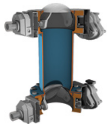
▲ Airlock / Double-Dump Assembly Two Roto-Disc valves are placed in series and are opened and closed independently, so pressure or vacuum is contained above or below the assembly
