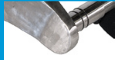
▲ Square shaft and dome holes are machined to exacting tolerances to provide a tight slip-fit that won't allow the actuator and dome to become decoupled.
